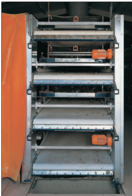
Manure removal end set with manure chute
