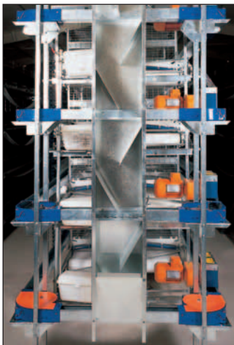
Cascade feed column prevents feed bridging
